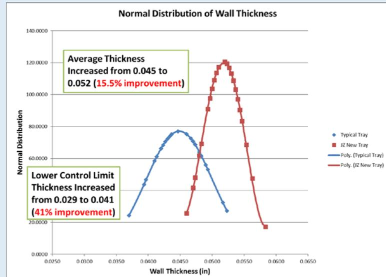
**Statistical analysis substantiating increased wall thickness**
